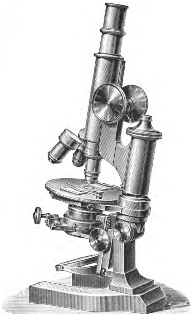
FIG. 14.—Leitz's Stand Ia., with a triple nose-piece and Abbe's condenser.
